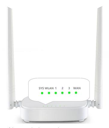
States of LED indicators of the router that is powered on
