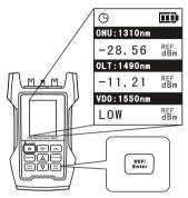
Setting reference is usually used before measuring the real network. It can wipe off the attenuation value which is not counted in the actual loss. Or it can be used in comparing with the pre-setting standard power.
