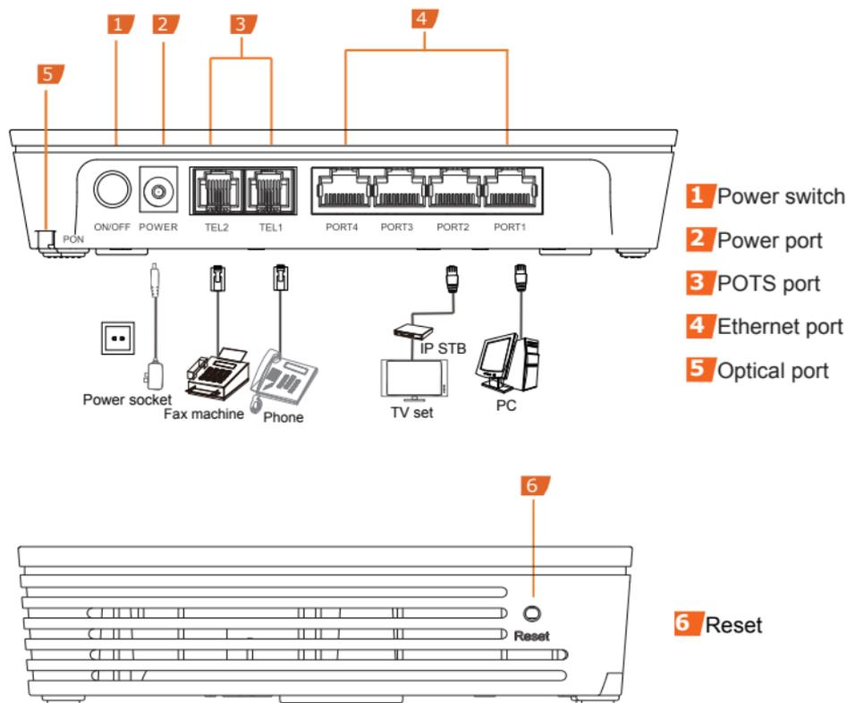
**Step 1** Use an optical fiber to connect the optical port on the ONT and the optical port on the wall.
