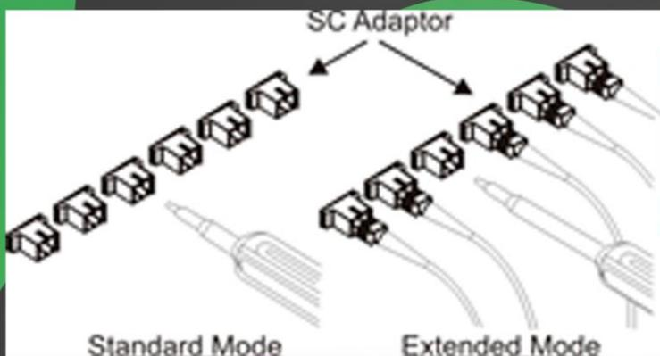
**3 - EMPURRE O INVÓLUCRO EXTERNO PARA LIMPAR A FACE FINAL DO CONECTOR SC, FAZENDO UM ZUMBIDO INDICANDO QUE O PROCESSO DE LIMPEZA TERMINOU E FECHANDO A TAMPA APÓS O USO.**
